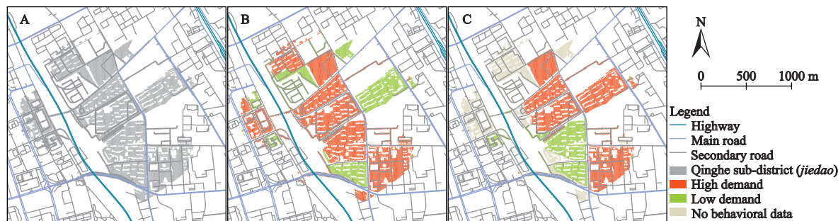
Fig. 7 Delineated life circle in the Dangdai Chengshi Jiayuan (DDJY) community: (A) 15-min walking-accessible range; delineation result based on the (B) estimated demand and (C) actual demand
