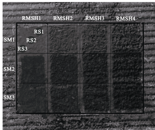
Fig. 1 Layout of the experimental area. SR1, SR2, SR3 are spectral reflectance measured areas in each sub-regions. RMSH1, RMSH2, RMSH3, RMSH4 are four surface roughness levels, SM1, SM2, SM3 are three soil moisture levels
