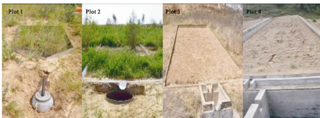
Plot 1: 1.2 m × 1.2 m; Plot 2: 2 m × 4 m; Plot 3: 5 m × 10 m; Plot 4: 5 m × 20 m; location: semi-arid loess hilly area in China Splash erosion is reduced by effective plant coverage in plots 1 and 2. Meanwhile, with the shortness of plot length, overland flow did not occur in these two plots. On the contrary, rill and ephemeral gully erosion were well developed due to the erosive rainfall, bare soil, and long plot length in Plot 4.
