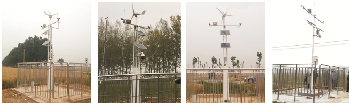
Fig. 2 Four IOT stations for monitoring of factors influencing SOC in experimental area
