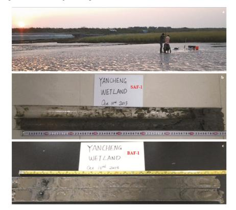
**Fig. 2** A photo showing sampling site scene at Yancheng coastal wetland and core sampling in the field (a), and photos showing the sediment cores of SAF-1 (b) and BAF-1 (c) that PVC pipes were cut in half to show the lithologic character in laboratory
