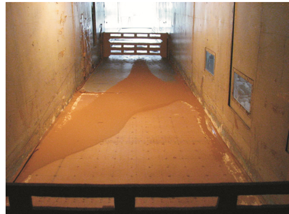
Fig. 10 Sand deposition in sand fence (SF) in wind tunnel experiments
