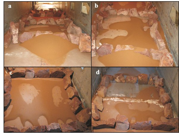
Fig. 8 Sand deposition in stone checkerboard barriers (SCBs) in wind tunnel experiments. a, before first SCB; b, inside first SCB; c, inside second SCB; and d, inside third SCB
